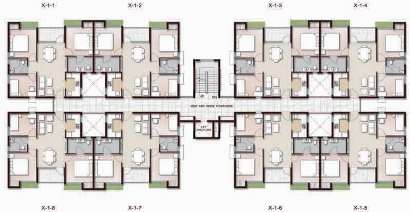
3 Bed Typical Block Plan (S+4), 1st to 4th
